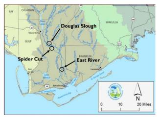
The intent of this project is to remove sand, logs, and other debris from a series of sloughs to increase water flow and hydrologic connectivity of sloughs with the main stem of the Apalachicola River in hopes of supporting floodplain recovery. Georgia offered as a metaphor the problem of clogged arteries in humans that inhibit blood circulation.
