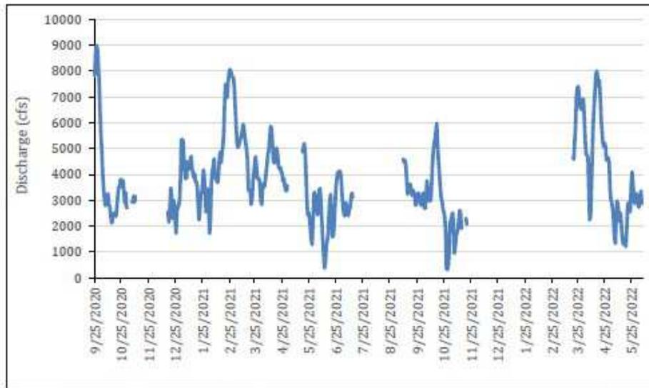
Figure 5: Flows Measured at USGS Station 0298308085143700 (IWW EAST OF GULF CO CANAL NEAR PORT ST JOE, FL. Positive flows indicate flows towards the Gulf County Canal and St. Andrew Bay.
